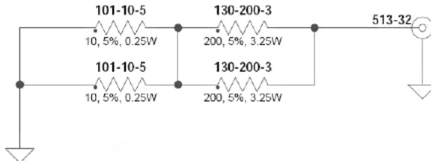
**Figure B-2.** Anritsu Model T3377 Low Current Test Fixture (for Option 10)
