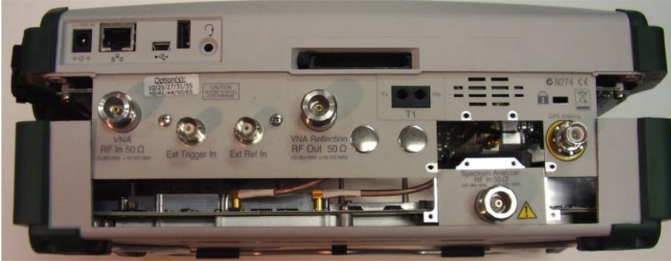
**Figure 3-6.** Separating the Case
