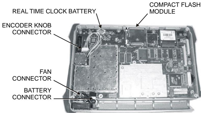
Figure 3-9. RTC Battery Location
