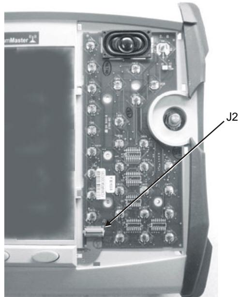
**Figure 3-12.** Connector J2 between the Keypad and the Flexible Switchpad
