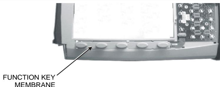
**Figure 3-11.** Function Key Membrane
